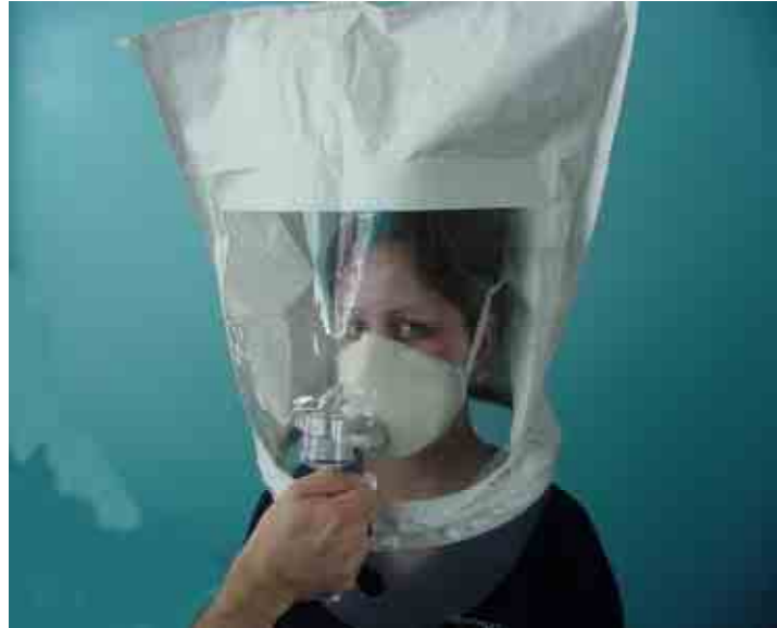
Fig. 7 Qualitative fit test - taste
